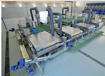
SF:6000 filters treating 1,650 m 3 /h SF:6000 Filter behandeln 1.650 m 3 /h
