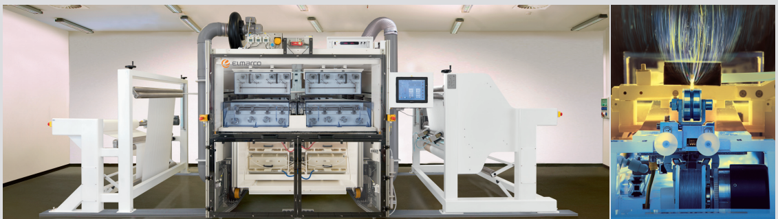
High volume production equipment – NS Production Line 1600 (left) Electrospinning process (right)
